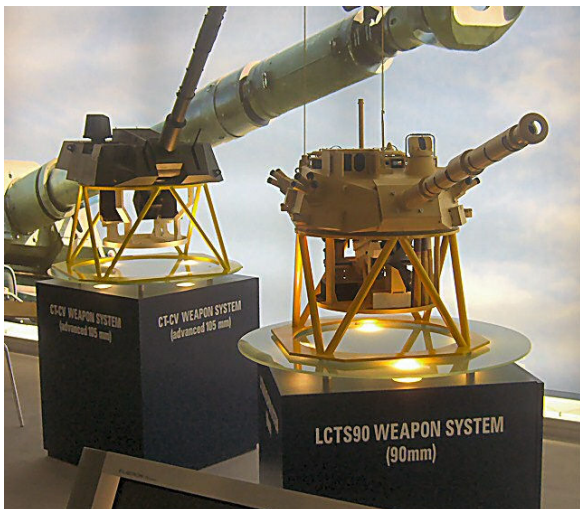
1:4 Scale LCTS 90mm and CT-CV 105mm Turrets
